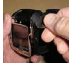
Fig. 97 - REMOVING THE BATTERY COVER
